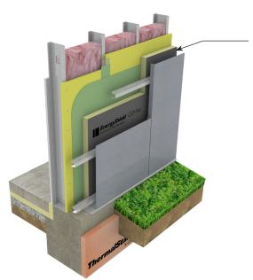
EnergyShield® CGF Pro facers add durability to help protect the integrity of the CI during the construction process.
