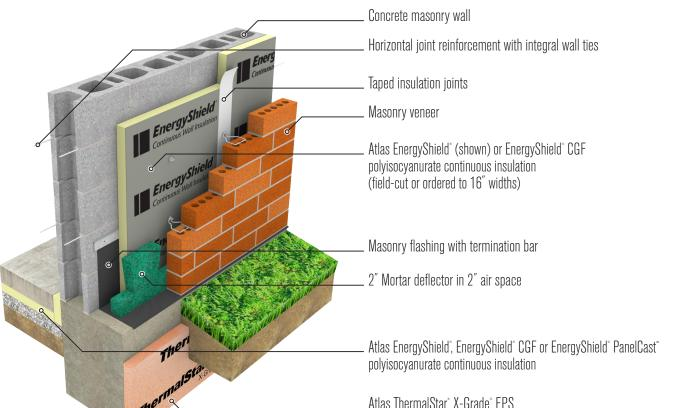
rigid continuous insulation at foundation
