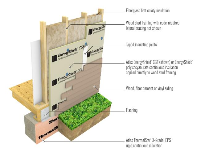
**Note:** Approved lateral bracing methods such as 1"×4" wood let-in-bracing, metal strap cross bracing, inset shear panels and structural sheathing at corners and at regular intervals must be used when polyiso foam is applied directly to wood stud framing. Consult architect, engineer, local code and code official for most appropriate solution.
