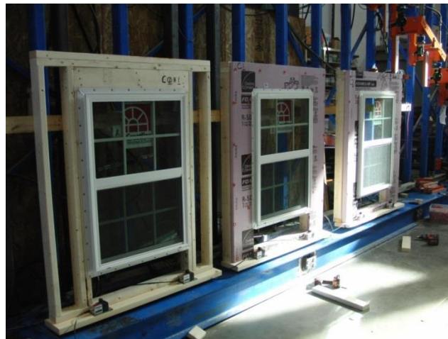
Photo 1: Long-Term Deflection under Self-Weight Testing
