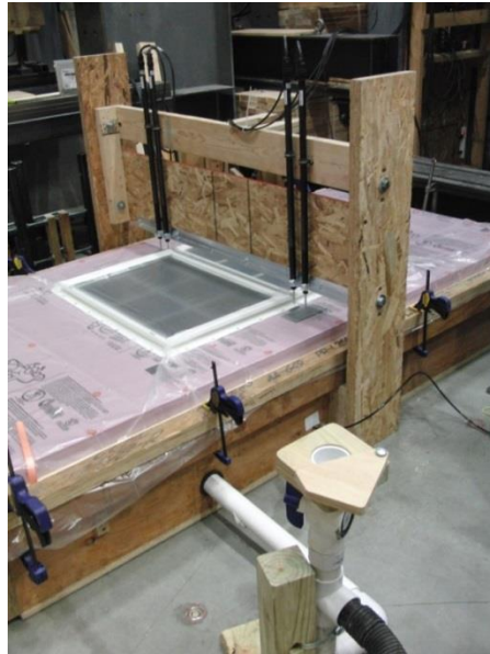
Photo 3: Wind Pressure Loading Test Setup
