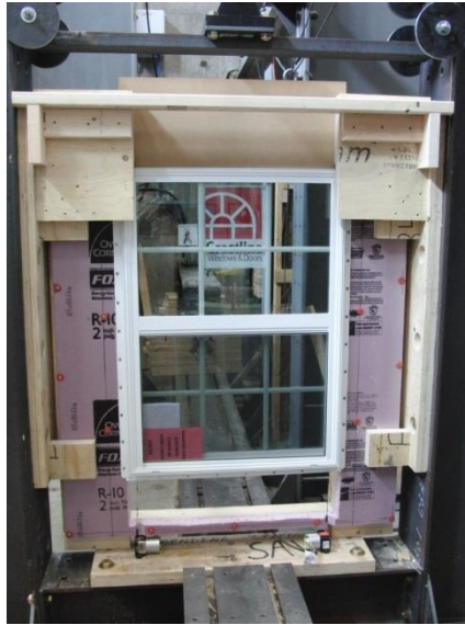
Photo 2: Structural Loading – Fastener/Flange Capacity
