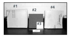
All samples were initially  $12" \times 12"$  and exposed to 200°F for 7 days:
