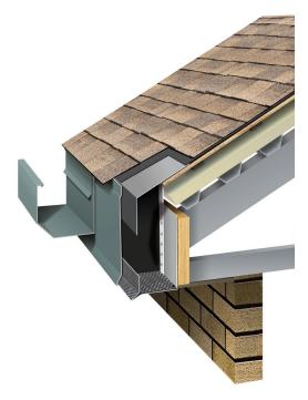
The above image shows the components of the Techni-Flo® EV. Proper installation is required to achieve optimal airflow through the eave and to maintain warranty coverage. Go to www.atlasroofing.com for further installation instructions.
