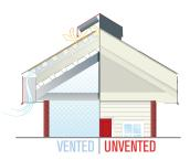
The Techni-Flo® RV is just one part of the Techni-Flo® Engineered Ventilation system. When combined with the Techni-Flo® EV and ACFoam® CrossVent and Atlas® Nail Base Fasteners, it creates a state-of-the-art ventilation system specifically designed to create consistent air intake and exhaust under the roof covering. Properly designed and engineered ventilation through the roof system is essential for roof system durability in both commercial and residential steeped-sloped roofing systems.
