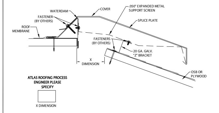
CAUTION! INSTALLERS SHALL WEAR PROTECTIVE EYE WEAR TO PREVENT INJURY. DO NOT OVERDRIVE FASTENERS, AS STRIPPING CAN OCCUR AT HIGH DRIVER TORQUE. RECOMMENDED DRIVING TOOL: 600 - 800 rpm ELECTRIC DRILL EQUIPPED WITH DEPTH-SENSING NOSE-PIECE TO PREVENT DRIVING AND STRIPOUT. DO NOT USE IMPACT TYPE TOOL.
