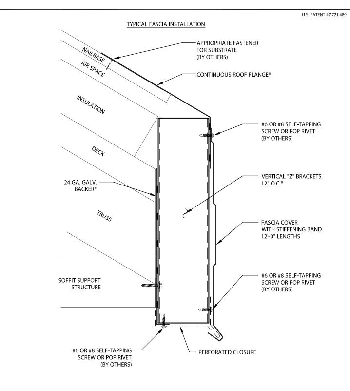
\*BACKER ASSEMBLY (FACTORY ASSEMBLED CONTINUOUS ROOF FLANGE, 24 GA. GALV. BACKER, AND VERTICAL "Z" BRACKETS 12" O.C.) TYPICAL STIFFENING BAND USED FOR TECHNI-FLO FASCIA SYSTEMS (VENTED NAILBASE VERSION)
