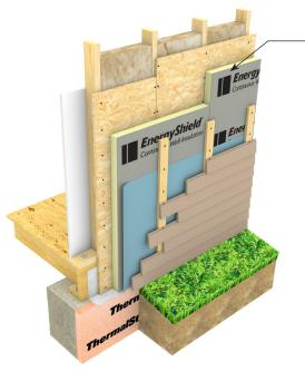
EnergyShield<sup>®</sup> NH combines high R-value, durable foil facers and water resistive attributes suitable for a variety of continuous insulation CI applications.
