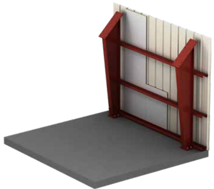
Illustration 2 Engineered Metal Building Wall
