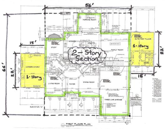
STEP 1: Determine Dimensions of Two-Story and One-Story Portions of 1<sup>st</sup> Story Floor Plan
