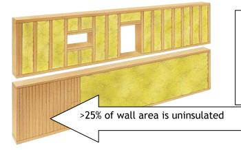
In a typical framed wall with <u>only</u> cavity insulation, over 25% of the wall area is uninsulated wood framing, forming a large thermal short. By installing foam insulation sheathing over the studs, a full insulation 'envelop' provides energy efficiency as well as a moisture resistant barrier for the wall system - something structural panels are unable to provide.
