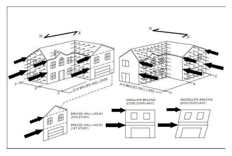
Figure 1: Wall Bracing and Racking Forces
