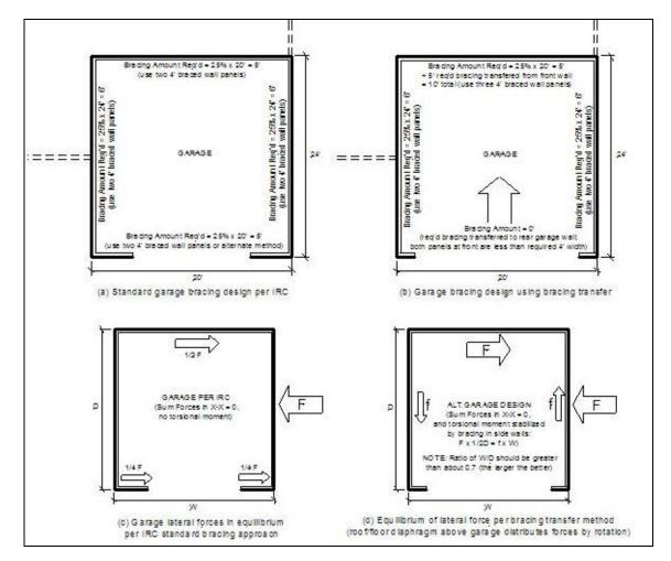
Figure 18: Bracing Transfer
