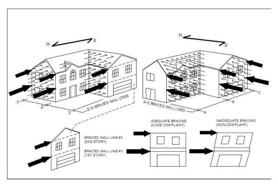
Figure 17: Example house plan for bracing length calculation
