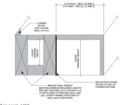
For SI: 1 foot = 305 mm. 1 pound = 4.448 N. Figure 15: BRACED WALL LINE WITH CONTINUOUS SHEATHING—FIRST BRACED WALL PANEL AWAY FROM END OF WALL LINE WITH HOLD-DOWN (IPC Eigure PEO2 10 4 4 (5)
