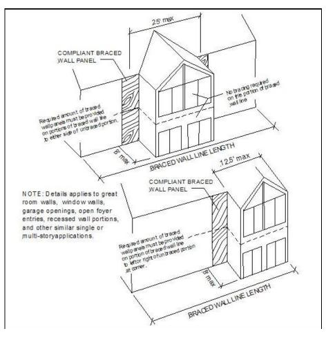
Figure 10: Limits for Large Openings in Braced Wall Lines with Intermittent Bracing
