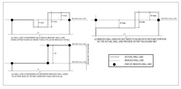
Figure 2: Braced Wall Line Layout Rules (Offsets and Ends)
